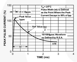
Figure 3. Pulse Waveform
