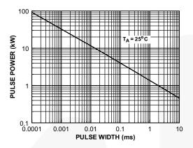
Figure 1. Peak Pulse Power Rating Curve
