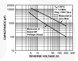
Figure 4. Junction Capacitance
