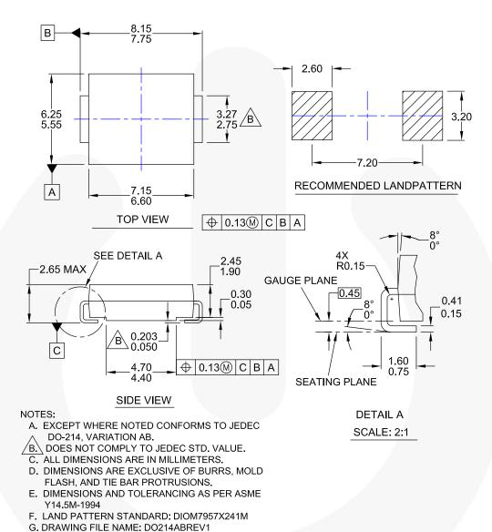
Figure 6. 2-LEAD, SMC, JEDEC DO-214, VARIATION AB (ACTIVE)
