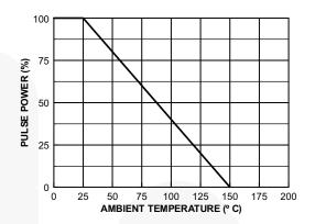
Figure 2. Pulse Derating Curve
