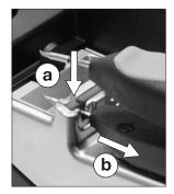
Place the tool in the extractor and pull to remove the cartridge.
