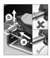
Follow the same steps conversely. It is essential to insert the cartridges as far as the ring for a proper connection.
