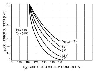
Figure 4. Reverse–Bias Switching Safe Operating Area
