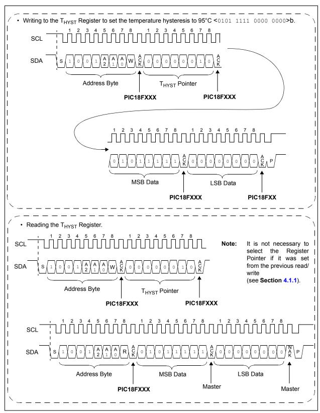
**FIGURE 5-5:** Timing Diagram for Writing and Reading from the Temperature Hysteresis Register (See Section 5.3.3 "Temperature Hysteresis Register (T<sub>HYST</sub>)").
