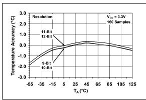
**FIGURE 2-3:** Average Temperature Accuracy vs. Ambient Temperature,  $V_{DD} = 3.3V$ .
