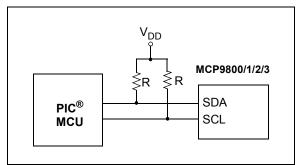
FIGURE 6-1: Pull-up Resistors on Serial Interface.
