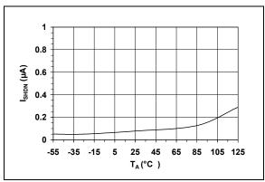
FIGURE 2-6: Shutdown Current vs. Ambient Temperature.
