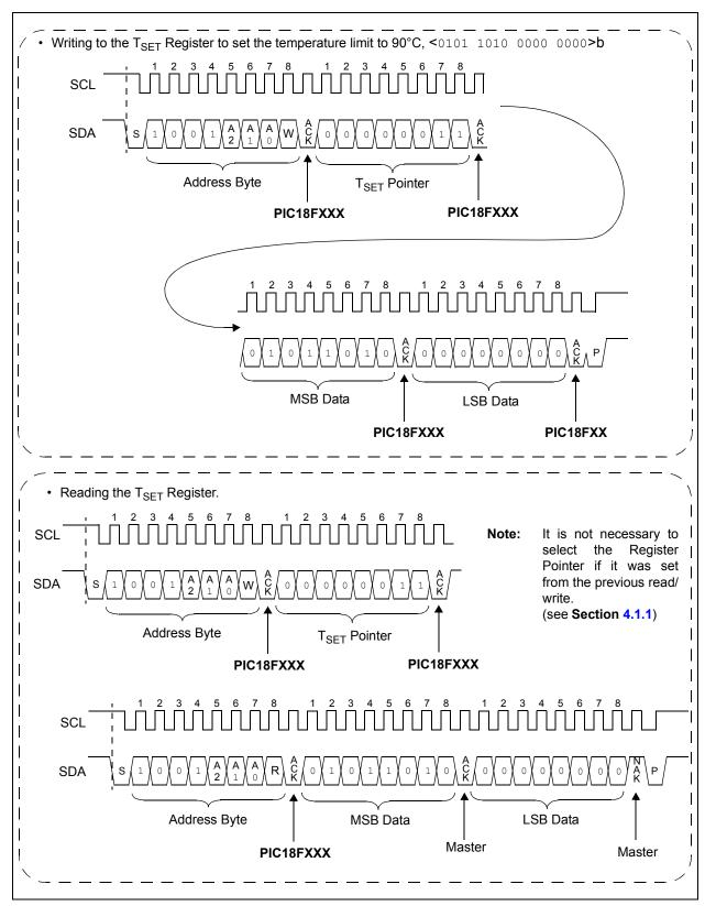
**FIGURE 5-6:** Timing Diagram for Writing and Reading from the Temperature Limit-set Register (See Section 5.3.4 "Temperature Limit-Set Register (T<sub>SET</sub>)").
