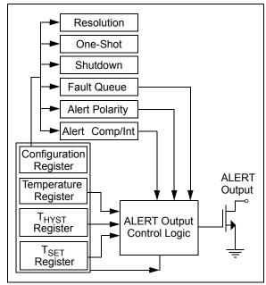
FIGURE 5-2: Register Block Diagram.
