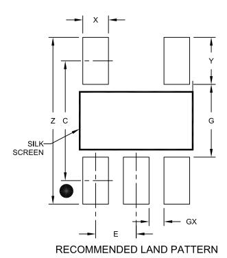
Units **MILLIMETERS** Dimension Limits MIN NOM MAX Contact Pitch 0.95 BSC Е Contact Pad Spacing С 2.80 Contact Pad Width (X5) Χ 0.60 Contact Pad Length (X5) Υ 1.10 Distance Between Pads G 1.70 Distance Between Pads GX 0.35 Overall Width 3.90 Z
