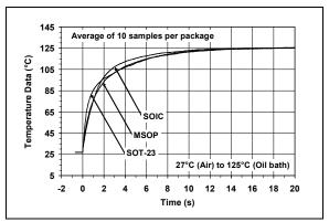
**FIGURE 2-9:** MCP980X Thermal Response vs Time.
