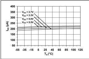
FIGURE 2-5: Supply Current vs. Ambient Temperature.
