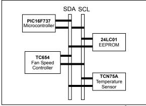
**FIGURE 6-2:** Multiple Devices on  $l^2C^{TM}$  Bus.
