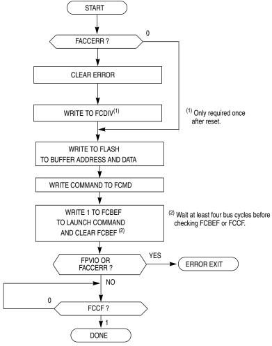
Figure 4-2. FLASH Program and Erase Flowchart
