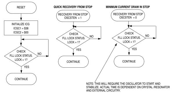
Figure 10-14. ICG Initialization for FEE in Example #1
