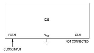
Figure 10-4. External Clock Connections
