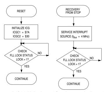
Figure 10-15. ICG Initialization and Stop Recovery for Example #2
