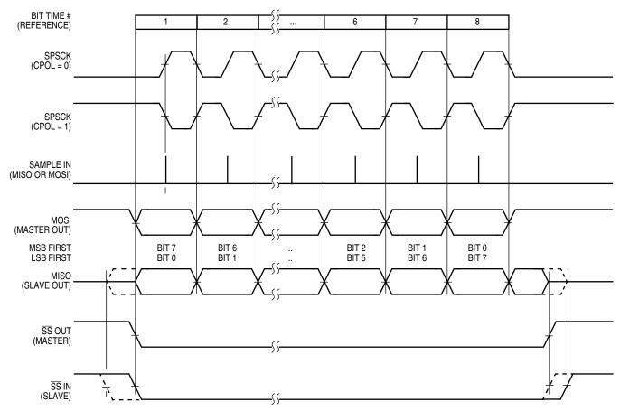
Figure 14-11. SPI Clock Formats (CPHA = 0)
