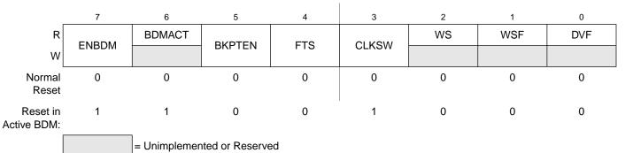
Figure 16-5. BDC Status and Control Register (BDCSCR)
