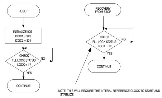
Figure 10-16. ICG Initialization and Stop Recovery for Example #3
