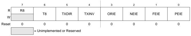
Figure 13-10. SCI Control Register 3 (SCIxC3)
