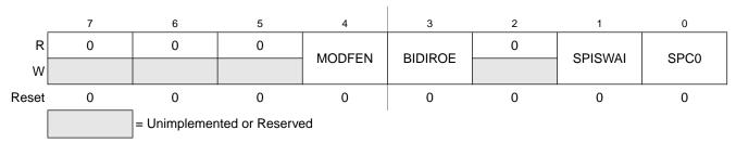
Figure 14-6. SPI Control Register 2 (SPIC2)
