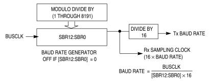
Figure 13-12. SCI Baud Rate Generation
