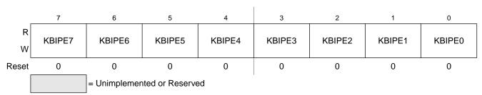
Figure 12-4. KBI Pin Enable Register (KBIPE)
