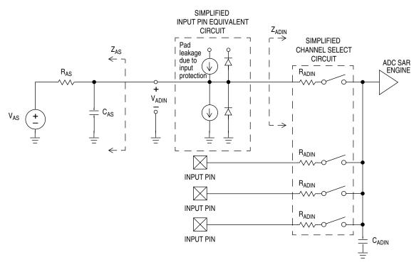
Figure A-8. ADC Input Impedance Equivalency Diagram
