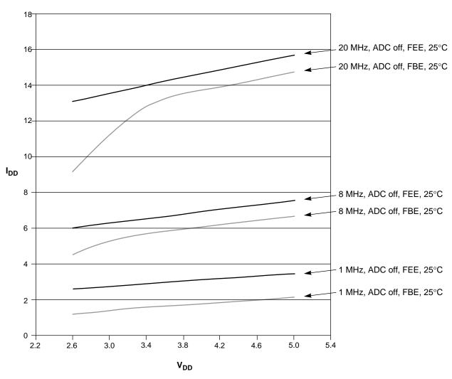
Note: External clock is square wave supplied by function generator. For FEE mode, external reference frequency is 4 MHz Figure A-5. Typical Run  $I_{DD}$  for FBE and FEE Modes,  $I_{DD}$  vs.  $V_{DD}$
