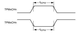
Figure A-14. Timer Input Capture Pulse
