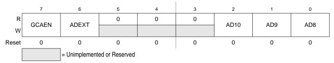
Figure 11-8. IIC Control Register (IICC2)
