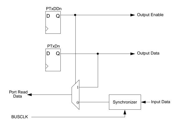
Figure 6-1. Parallel I/O Block Diagram
