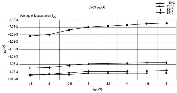
Figure A-7. Typical Stop3 I<sub>DD</sub>
