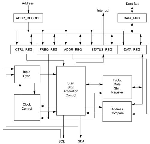
Figure 11-2. IIC Functional Block Diagram
