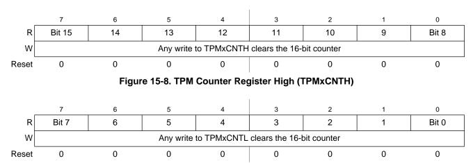
Figure 15-9. TPM Counter Register Low (TPMxCNTL)
