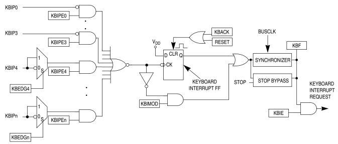
Figure 12-2. KBI Block Diagram
