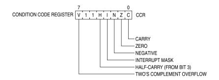
Figure 7-2. Condition Code Register
