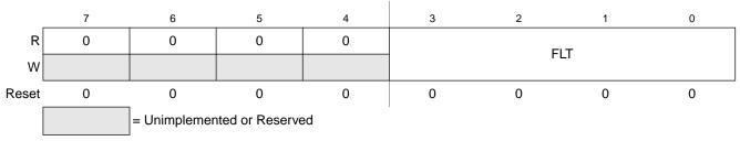
Figure 10-10. ICG Upper Filter Register (ICGFLTU)
