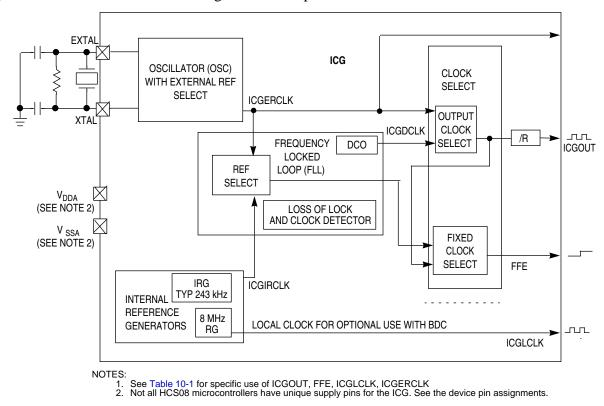
Figure 10-3. ICG Block Diagram
