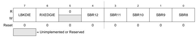
Figure 13-4. SCI Baud Rate Register (SCIxBDH)
