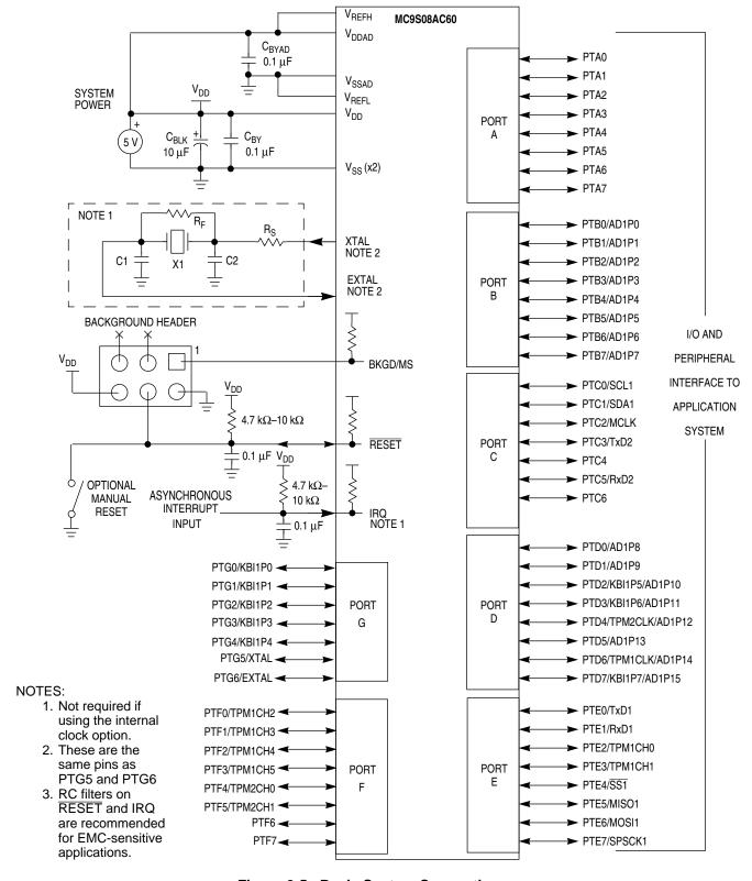
Figure 2-5. Basic System Connections
