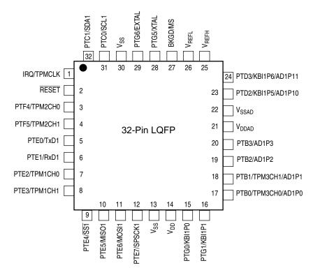
Figure 2-4. MC9S08AC60 Series in 32-Pin LQFP Package
