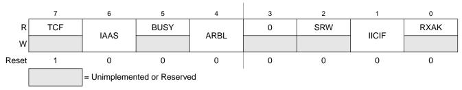
Figure 11-6. IIC Status Register (IICS)
