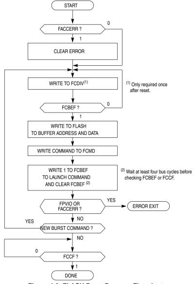
Figure 4-3. FLASH Burst Program Flowchart
