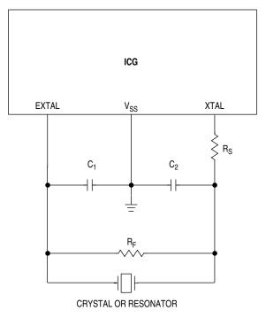
Figure 10-5. External Frequency Reference Connection
