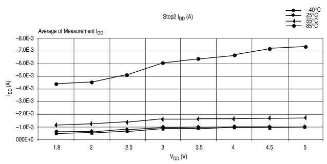
Figure A-6. Typical Stop 2 I<sub>DD</sub>
