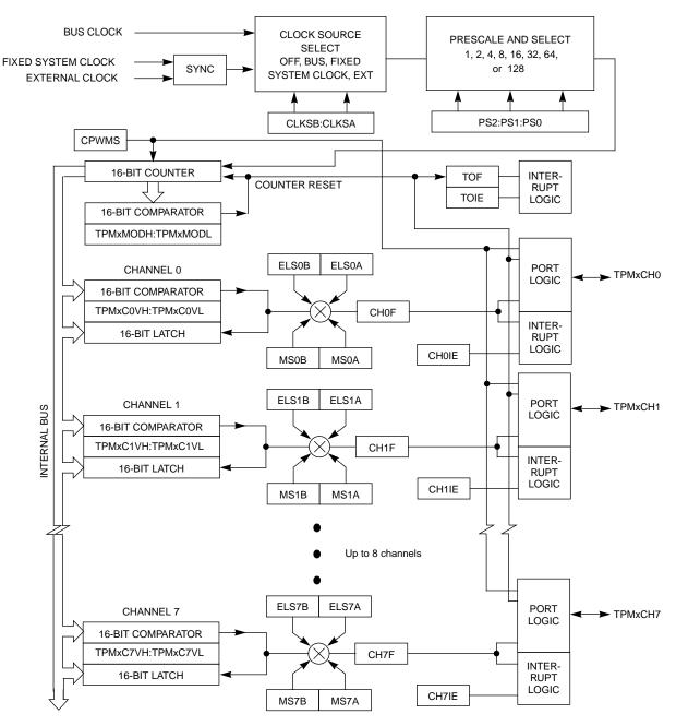
Figure 15-2. TPM Block Diagram
