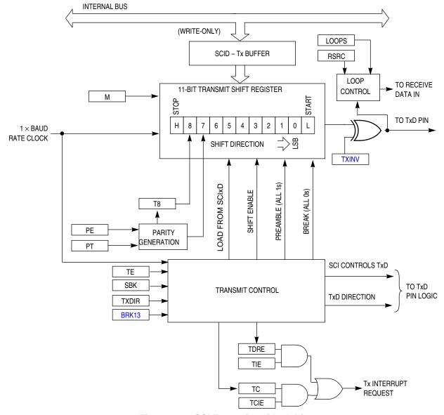
Figure 13-2. SCI Transmitter Block Diagram
