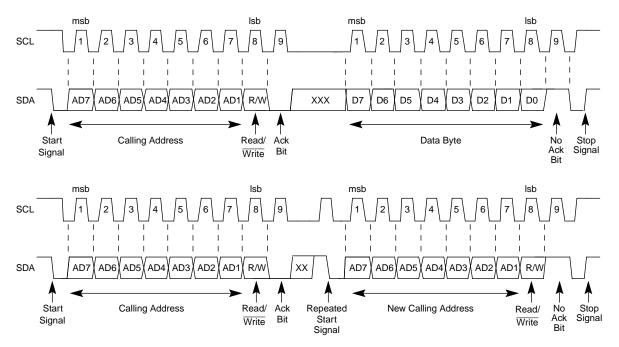
Figure 11-9. IIC Bus Transmission Signals
