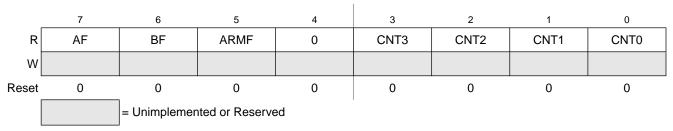
Figure 16-9. Debug Status Register (DBGS)
