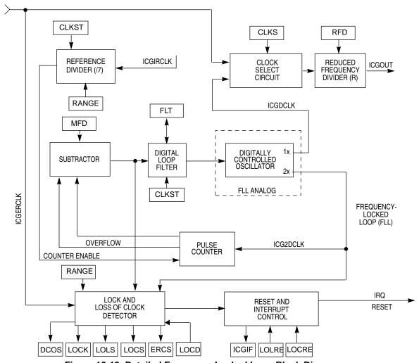
Figure 10-13. Detailed Frequency-Locked Loop Block Diagram
