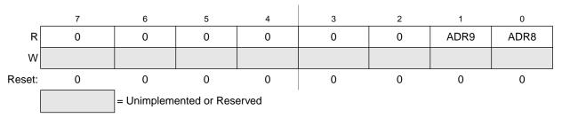
Figure 9-6. Data Result High Register (ADCRH)
