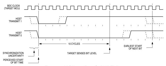
Figure 16-2. BDC Host-to-Target Serial Bit Timing
