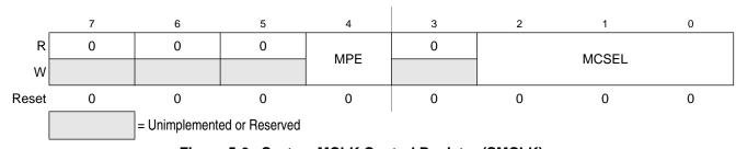
Figure 5-6. System MCLK Control Register (SMCLK)
