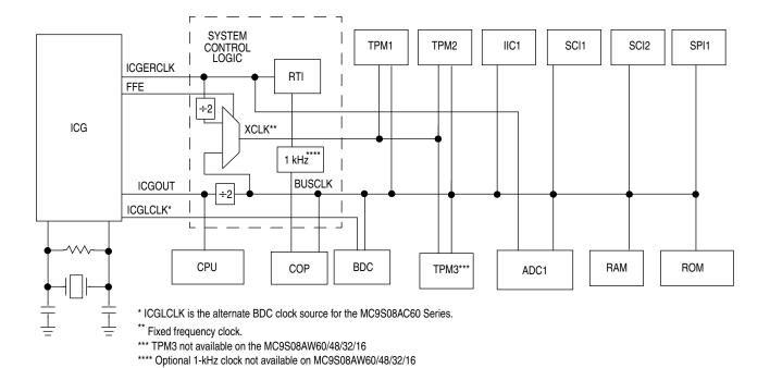
Figure 10-1. System Clock Distribution Diagram
