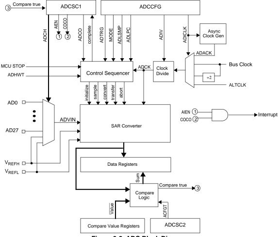
Figure 9-2. ADC Block Diagram
