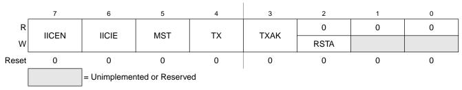
Figure 11-5. IIC Control Register (IICC1)
