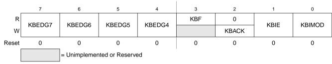
Figure 12-3. KBI Status and Control Register (KBISC)
