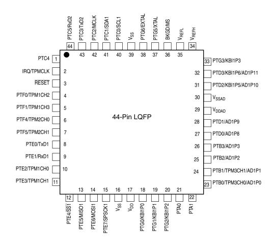
Figure 2-3. MC9S08AC60 Series in 44-Pin LQFP Package
