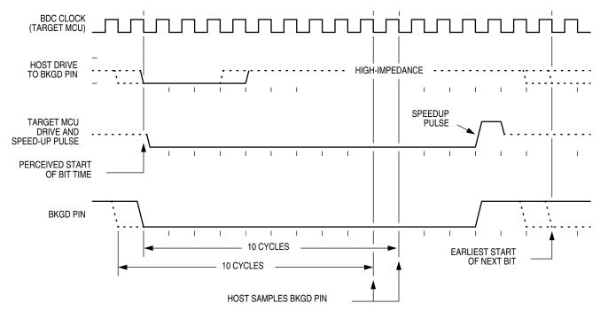
Figure 16-4. BDM Target-to-Host Serial Bit Timing (Logic 0)
