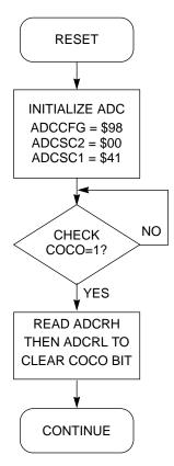
Figure 9-13. Initialization Flowchart for Example
