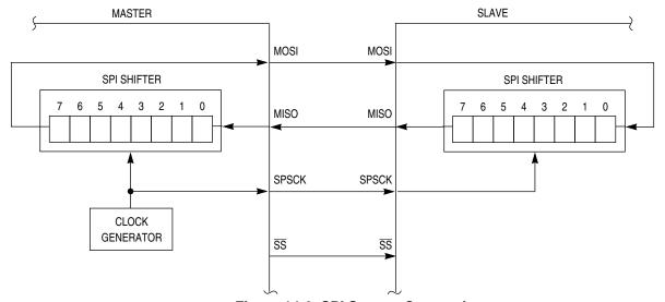
Figure 14-2. SPI System Connections
