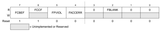
Figure 4-8. FLASH Status Register (FSTAT)
