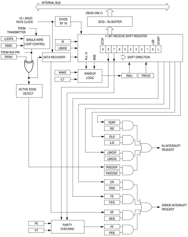
Figure 13-3. SCI Receiver Block Diagram
