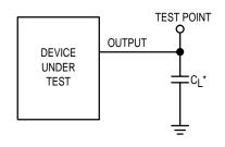
\* Includes all probe and fixture capacitance.
