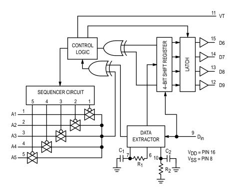
Figure 2. MC145027 Decoder Block Diagram
