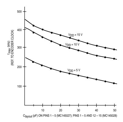
Figure 12. f<sub>max</sub> vs C<sub>layout</sub> — Decoders Only
