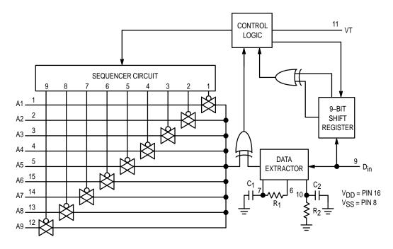
Figure 3. MC145028 Decoder Block Diagram
