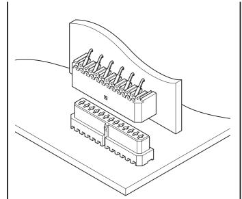
The JE connector is a compact, board-toboard connector only 6.8mm high and 3.6mm wide. Its mating part has a 1.25mm pitch, single row construction. High contact pressure dual beam fork contacts are combined with a housing lock mechanism to ensure a reliable connection.
