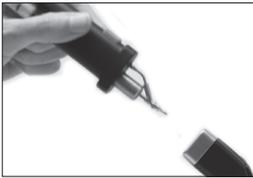
Lift tool from the stand and the tool tip will heat up to the selected temperature.
