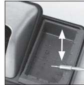
Tap gently to remove the excess of solder.
