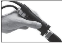
When the tool is in the stand, the temperature reduces to Sleep temperature (pre-set 260°C / 500°F).
