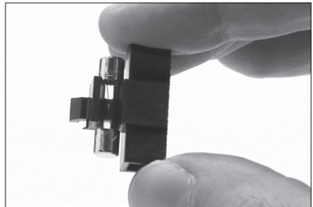
Press the new fuse into the holder and replace it in the station.
