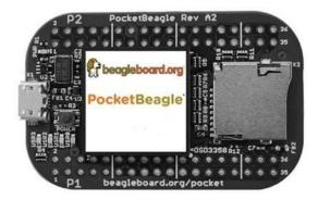
The newest BeagleBoard.org<sup>®</sup> board is PocketBeagle<sup>®</sup>, an ultra-tiny-yet-complete open-source USB-keyfob computer. PocketBeagle<sup>®</sup> features an incredible low cost, slick design and simple usage, making PocketBeagle<sup>®</sup> the ideal development board for beginners professionals alike.
