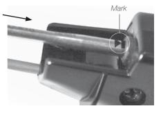
**Important:** Insert the cartridge as far as the mark for a correct connection.
