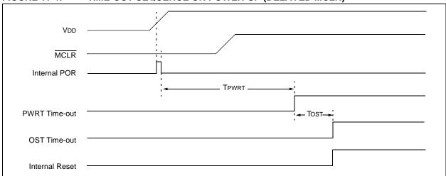
FIGURE 11-5: TIME-OUT SEQUENCE ON POWER-UP (DELAYED MCLR)
