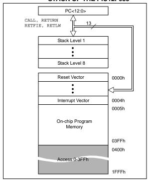
FIGURE 2-2: PROGRAM MEMORY MAP AND STACK OF THE PIC16F636
