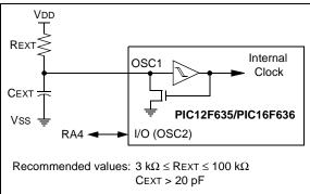
The RC oscillator frequency is a function of the supply voltage, the resistor (REXT) and capacitor (CEXT) values and the operating temperature. In addition to this, the oscillator frequency will vary from unit to unit due to normal threshold voltage. Furthermore, the difference in lead frame capacitance between package types will also affect the oscillation frequency or for low CEXT values. The user also needs to take into account variation due to tolerance of external RC components used.
