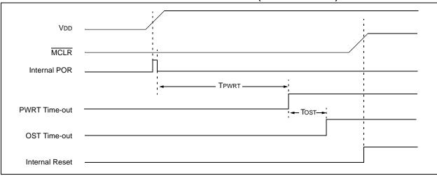
FIGURE 11-6: TIME-OUT SEQUENCE ON POWER-UP (MCLR WITH VDD)
