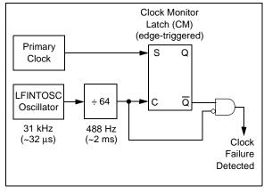
The FSCM function is enabled by setting the FCMEN bit in the Configuration Word register (Register 11-1). It is applicable to all external clock options (LP, XT, HS, EC, RC or I/O modes).
